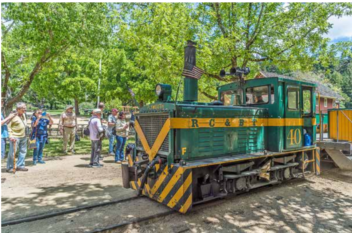
SWITCHER – Plymouth No. 40, a diesel-powered switch engine, is still in operation at the Roaring Camp & Big Trees Railroad.
