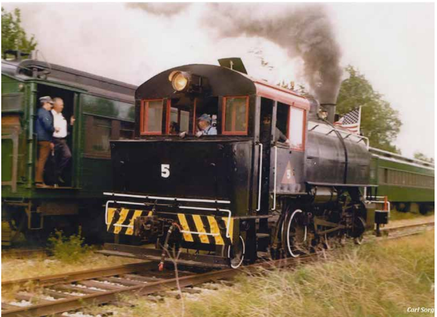
ON RUN-AROUND — This rare bunker-end view shows CO&E 2-4-2T No. 5 running around her train in the refuge at Ordill, Ill., on May 29, 1973.
