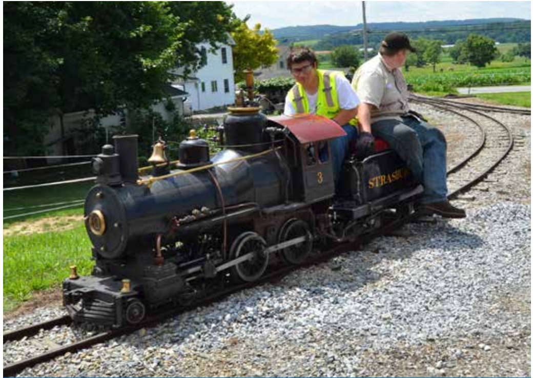
LIVE STEAMER — RailCamp attendee Joe Tibaldi opens the throttle of the Strasburg Rail Road’s 15-inch gauge Cagney live steam locomotive, under the tutelage of Strasburg employee Alex Merrill.
