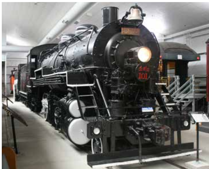
FROM KOREA — One of the earliest items in the museum's collection is the Army Pershing class 2-8-0, a 1917 Baldwin which was donated to the museum by the Republic of Korea in 1961.
