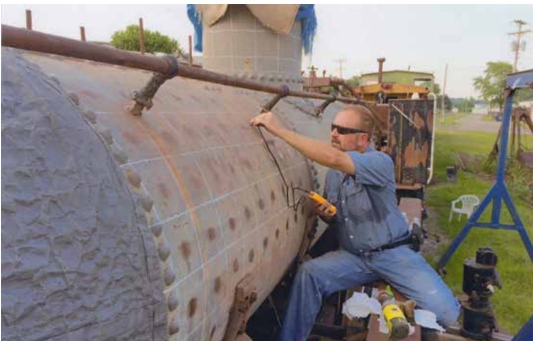
ULTRASOUND — Shawn Friedrich, a railroad volunteer, uses the ultrasound device to check the boiler measurements.
